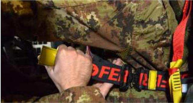
Figure 76 - Tightening the chest restraints
