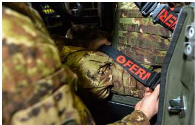
**Figure 85 - Attaching the groin restraint**
