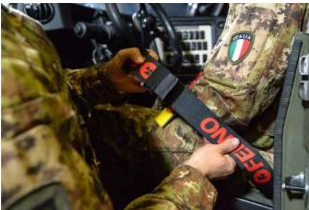
**Figure 81 - Extending the groin restraints**
