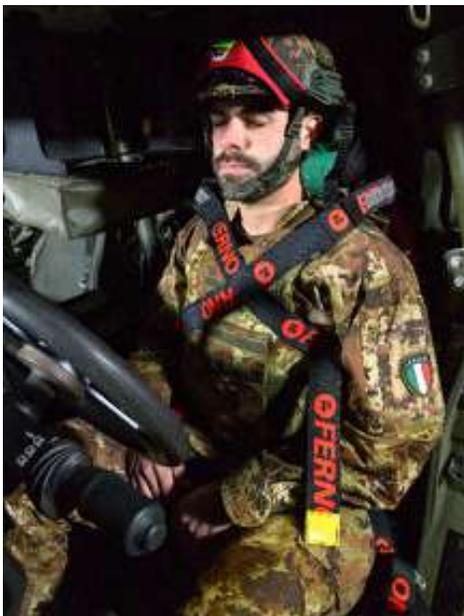
Figure 77 - Tightened chest restraints (Front view)
