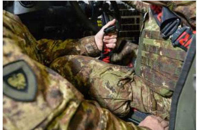
**Figure 83 - Tightening the groin restraint**
