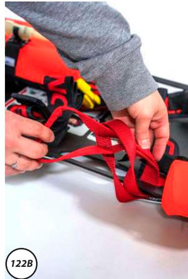
**Figure 122 - Fixing the auxiliary handles**
