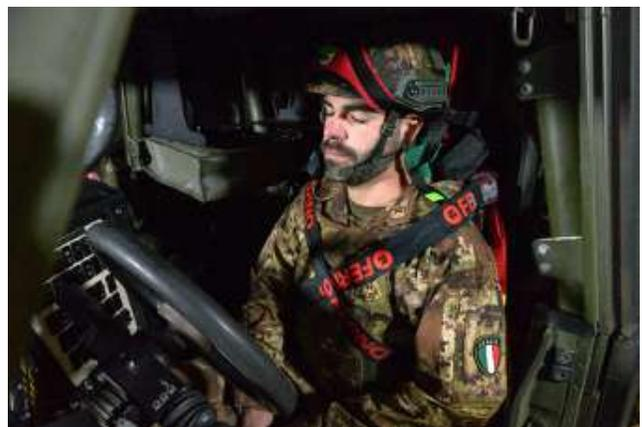
**Figure 75 - Correct position of the chest restraints**
