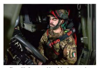
Figure 75 - Correct position of the chest restraints
