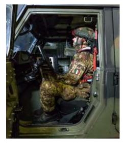
Figure 88 - Casualty secured to the XT MILITARY after all straps and restraints have been tightened
