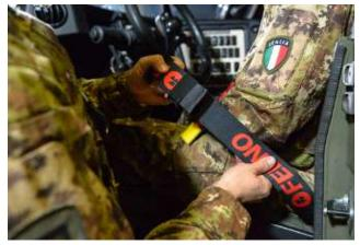
Figure 81 - Extending the groin restraints
