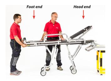
\*\* Figure 16 - Operators' positions to load the stretcher
