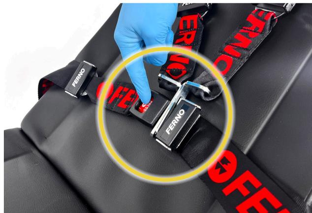
**Figure 45 - Four-point restraint opening**
