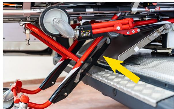
Figure 5 - Mechanical unlocking system for rear legs
