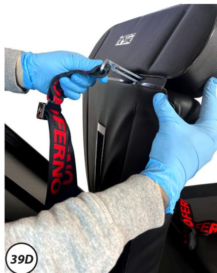
3. Insert the buckle into the loop (Figure 39B) and pass the buckle first through the slot in the ABS surface, and then through the slot in the mattress (if the mattress is not suitable, it must be replaced for the restraints to function correctly).
