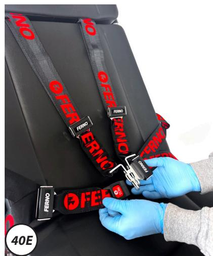
Figure 40 - Installing the lower section of the four-point restraint
