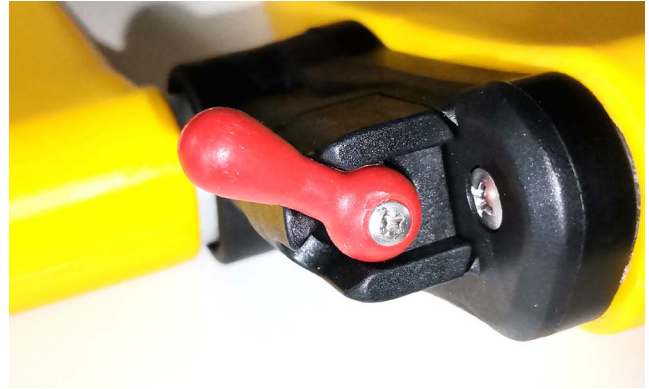
Figure 8 - Locking lever facing upwards
