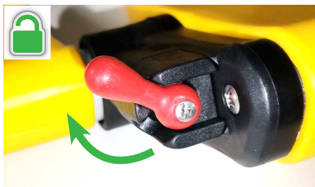
Figure 2 - Locking lever facing upwards: STRETCHER UNLOCKED
