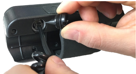
Figure 13 - Unplugging the connector
