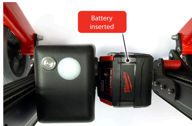
Battery fitted correctly
