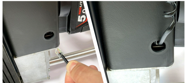
Figure 12 - Connecting the cable to the motor housing
