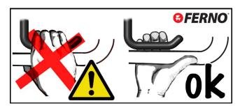
Label Front leg control handle: Correct hand positioning and handle operation.
