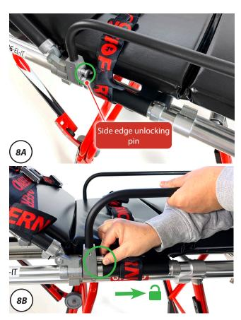
Figure 8 - A: Folding side edge unlocking pin B: Unlocking movement to lift or lower the side edges
