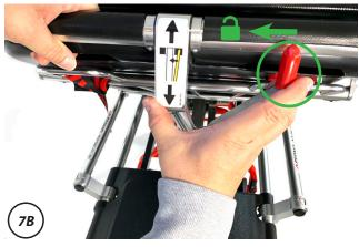
Figure 7 - A: Backrest B: Unlocking lever activation
