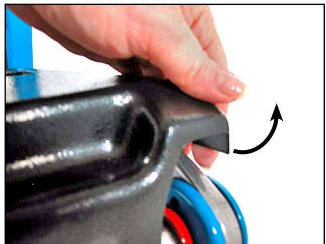
Figure 43 - Releasing a Corner of the Seat Panel
