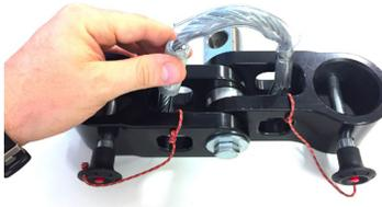
Pass the steel cable around the centre pin connecting the bipod head.
